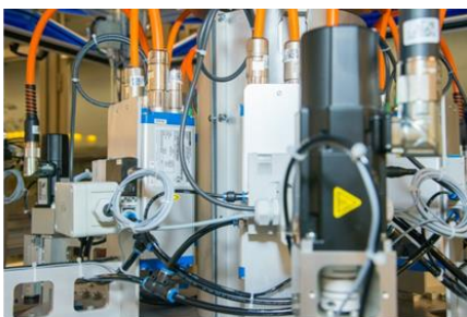
The decentralized AKD-N servo drives are positioned around the machine's central axis to save space.
