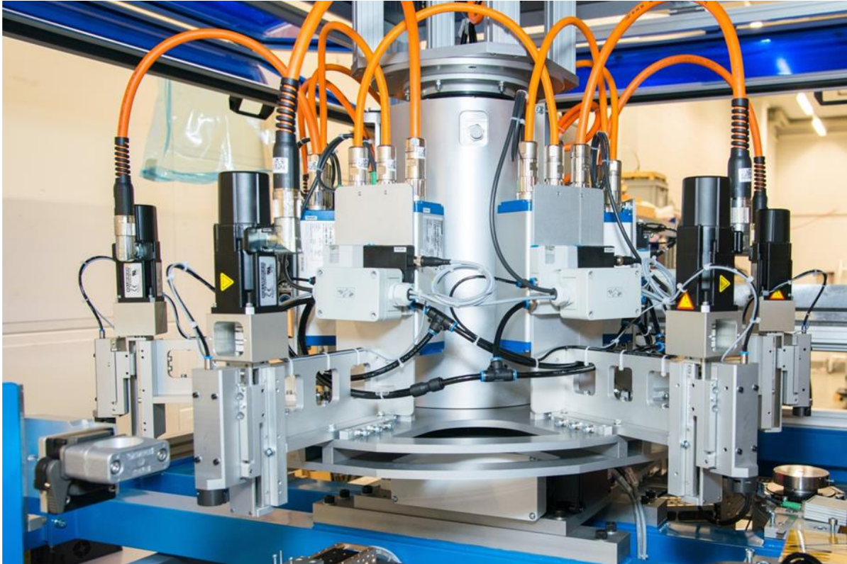
The servo motors from the KOLLMORGEN AKM series also travel along on the rotary indexing table.
